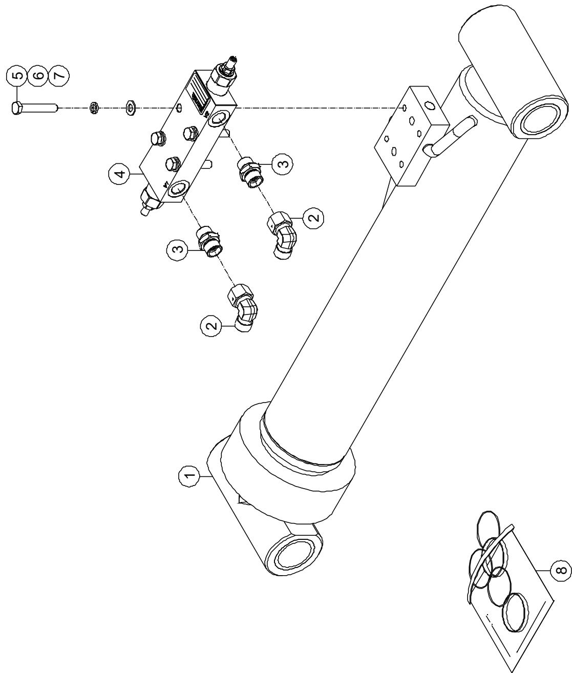
**5-5 JIB Leveling Cylinder Assembly (BT22ERT)**
